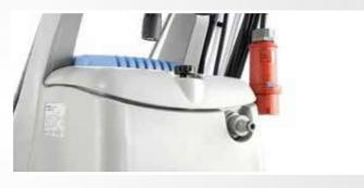
Always on the safe side: a float in a water box switches off the motor pump when a certain water level is reached and prevents pump damage in the event of Lack of water (on quadro models).
